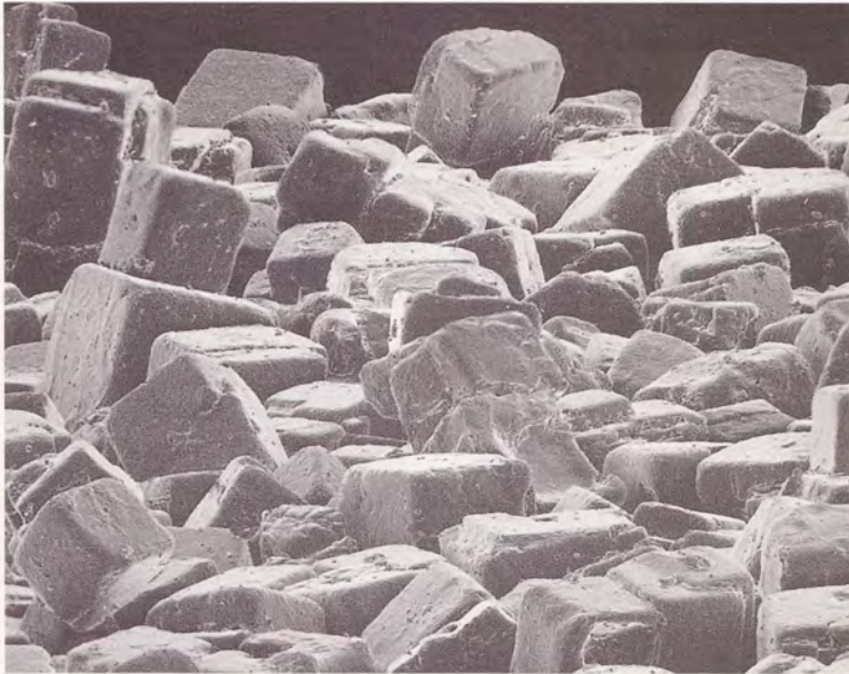
Fig. 6.10 Common table salt magnified 50 times by an electron microscope. The evident cubic structures reflect the underlying lattice structure.
